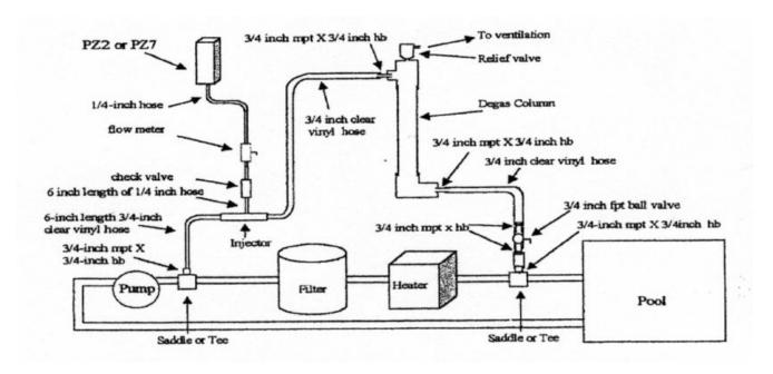
INSTALLATION IN STANDARD BYPASS CONFIGURATION
