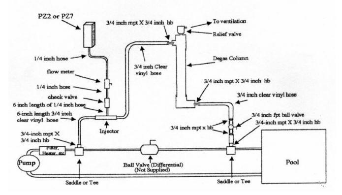
INSTALLATION AFTER FILTER, HEATER, ETC.
